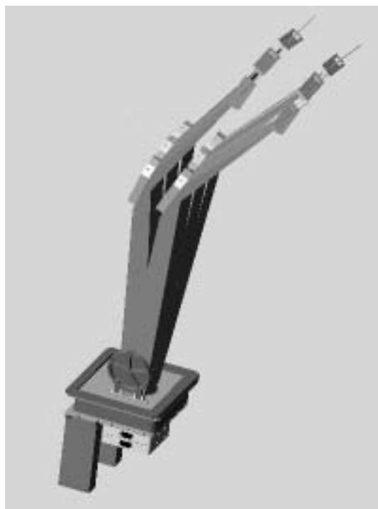
Figure 1: Light path of the six channels of the CHIPS spectrograph.
