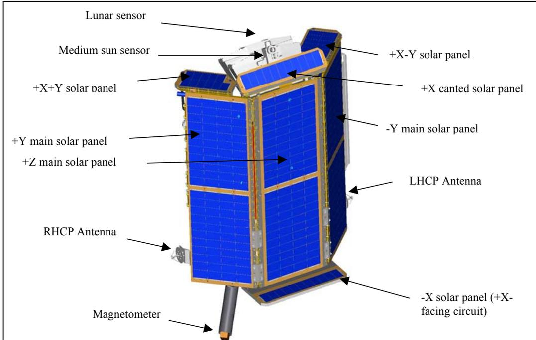
**Figure 4: View of CHIPSat +Z Direction (main solar arrays)**
