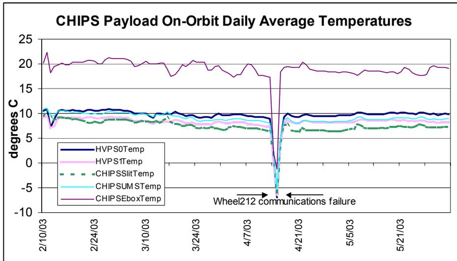
**Figure 9: Average daily temperatures of CHIPS instrument**
