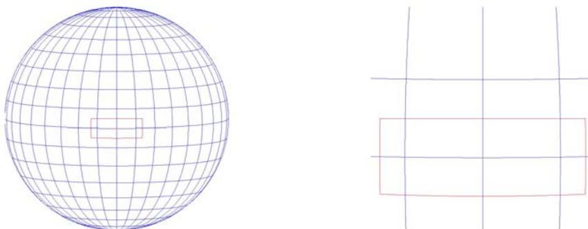
**Figure 2: View of Rectangular Chips FOV (5° x 26.6°) Projected onto a Celestial Sphere**
