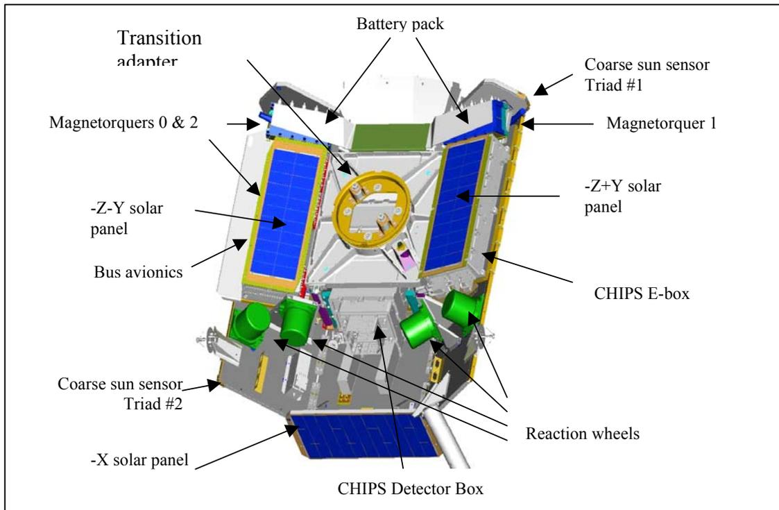
**Figure 5: View of CHIPSat -Z Direction (auxiliary solar arrays)**
