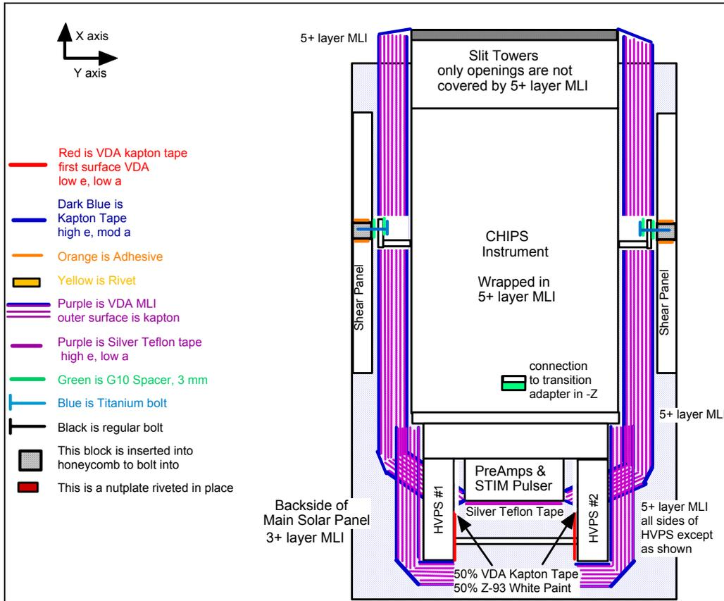
design of the CHIPS instrument from the +z direction.
